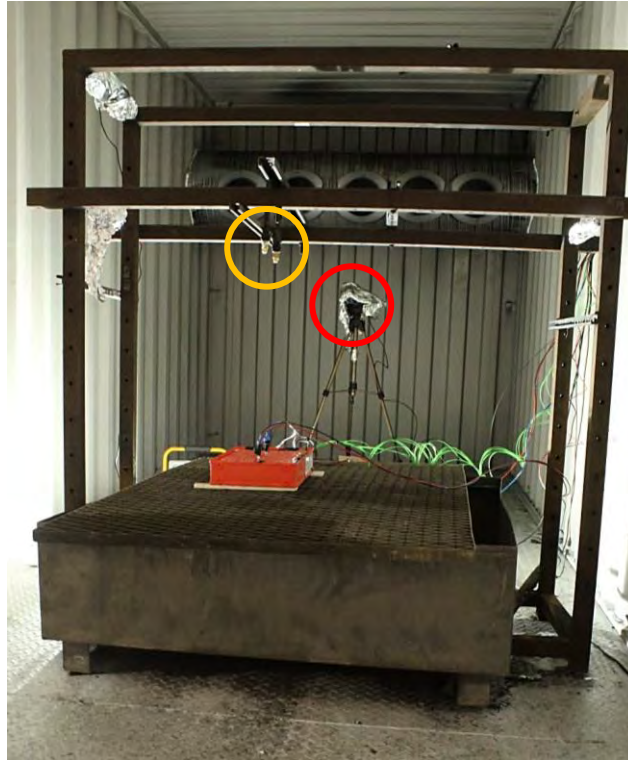
Figure 3: Overall setup of the experiment consisting of the battery in the lower area of the figure and the frame with the two nozzles for firefighting (yellow). The temperature of the entire system is measured using an infrared camera (red).
